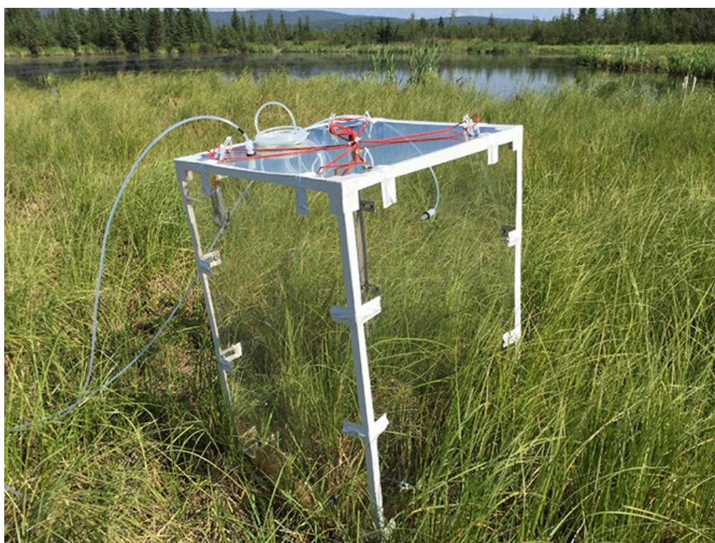
Figure 1. Photo of the custom-built chamber for measuring in situ trace gas fluxes from soil/vegetation and water surfaces (with flotation). The chamber (0.71 m x 0.71 m x 1.07 m = 0.533 m 3 ) provides adequate height to enclose emergent grasses and reeds. The chamber is connected by tubing to a Los Gatos Ultra-Portable Greenhouse Gas Analyzer capable of measuring trace gasses at 1 Hz in recirculating air. Photo courtesy C. Elder.
