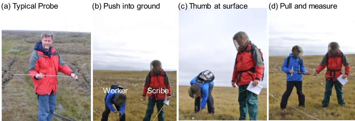
Figure 4: The active layer probe is a metal rod with a handle (a). To measure ALT, the worker pushes the probe into the ground to the permafrost layer (b), places a thumb on the metal rod at the ground surface (c), then pulls out the probe (d). The scribe measures the ALT with a tape measure and writes it down. Here, Lin Liu measures ALT along a survey line at Barrow, Alaska while Kevin Schaefer records the results in a notebook.
