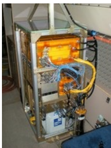
Figure 1. The Harvard QCLS (DUAL and CO 2 ) instrument package contains two optical assemblies and calibration systems and a common data system and power supply.
