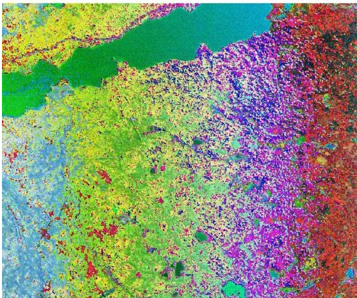
Figure 1. False color image of AVIRIS-Classic scene acquired over Waskesiu Lake, north of Prince Albert, Saskatchewan, Canada, on 1996-08-14. Flight: f960814t01, run 01, scene 07; latitude 53.9709, longitude -106.3295. Image shows channels 128 (1563 nm), 33 (666 nm), and 10 (458 nm) as red, green, and blue, respectively.
