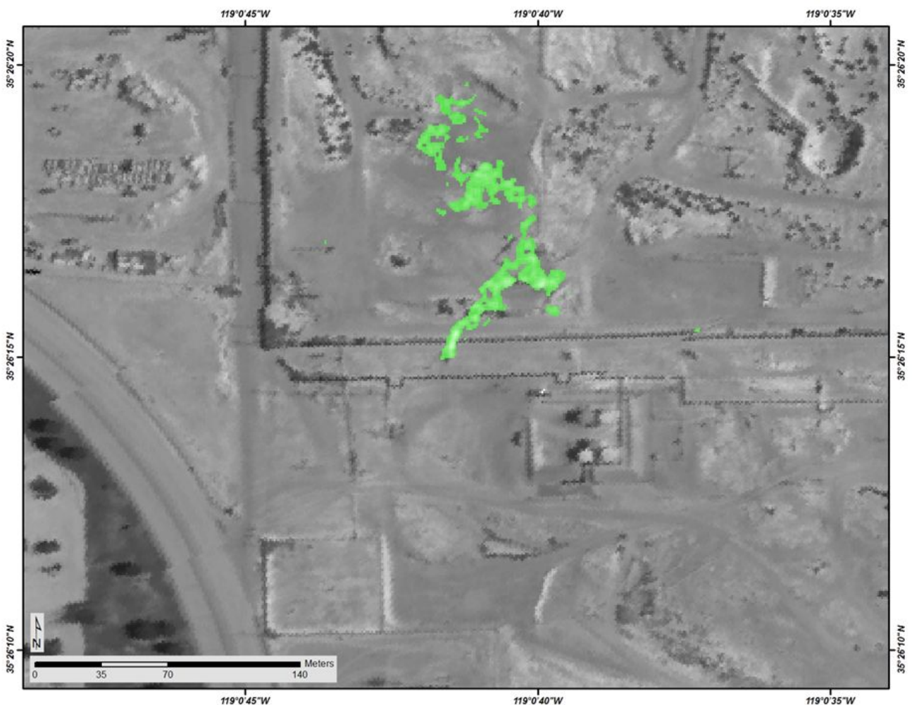
Figure 1. Methane detection signal (green) of pump jack leak at the Kern River oil field superimposed on the thermal radiance scene image. Image
