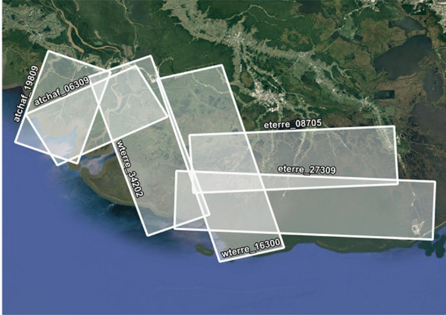
Figure 3. Spatial coverage of each UAVSAR flight line acquired during the 2021 Delta-X campaign. Map shows the Atchafalaya and Terrebonne Basins along the southern coast of Louisiana, USA.
