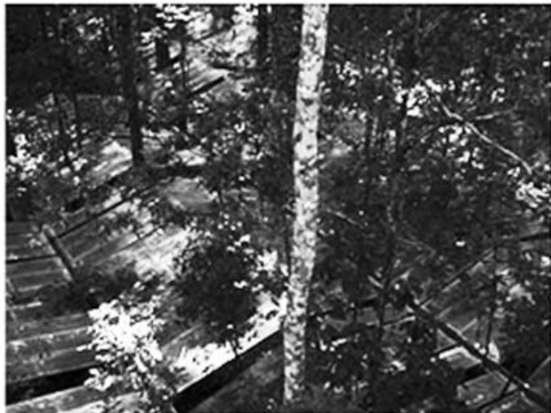
Throughfall exclusion panels, Tapajos National Forest. The throughfall exclusion panels drain into wooden gutters constructed in the forest understory. Photos from Nepstad et al., 2002.
