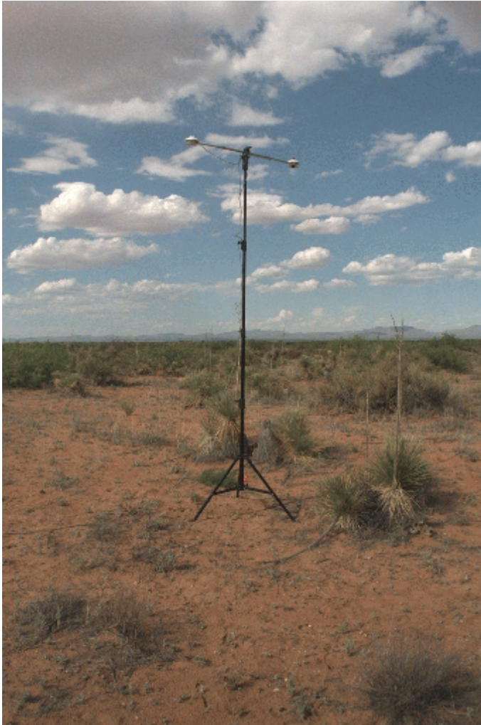
Figure 4.2: Albedometer instrument setup: the total shortwave and NIR broadband albedometers mounted on either end of a pole secured to the top of a black tripod at a height of approximately 4 metres above the surface. The albedometer mounting was replaced by the camera with a fish eye lens for the acquisition of hemispherical photographs from the same height as the albedo measurements. Photograph taken by Paul Hobson (University of Wales, Swansea).
