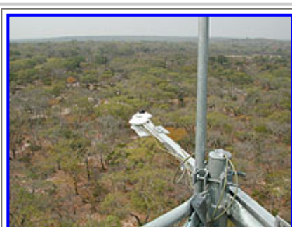
The CM14 Albedometer, a single body instrument with both an upward- and downward-looking pyranometer, on the Mongu tower.
