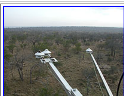
The CM14 Albedometer, the 'red dome' (NIR) and 'clear dome' sensors (left), and the second 'clear dome' sensor (right), on the Skukuza tower.
